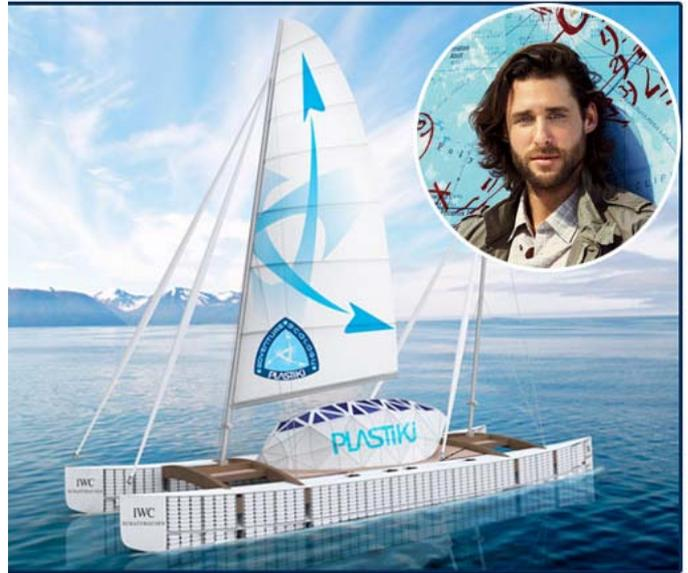
A unique plastic recyclable material made from srPET makes up her superstructure. The mast is reclaimed aluminium irrigation pipe and the sail is hand-made from recycled PET cloth.
